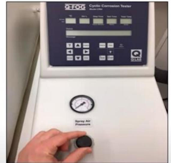
Fog Spray Air pressure 12-16 psi
