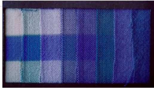
Blue Wool ISO textile test timing
