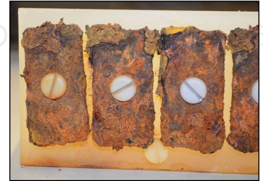
Mass-Loss Coupons Widely used in corrosion testing
