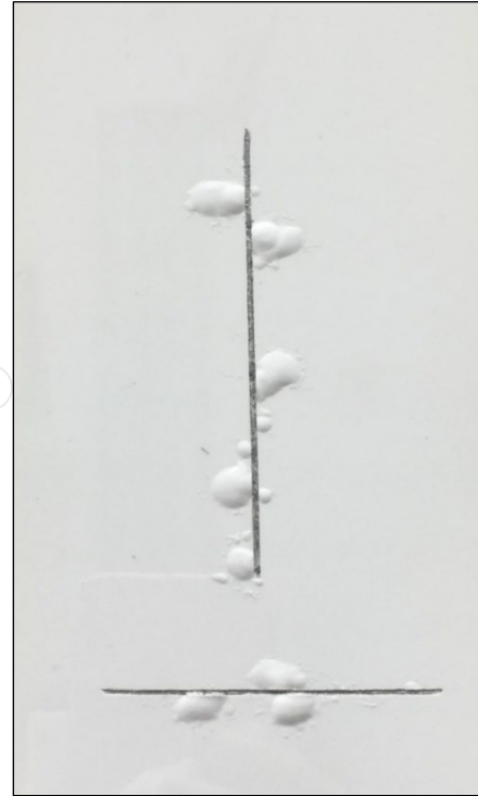
Corrosion morphology – Type D
