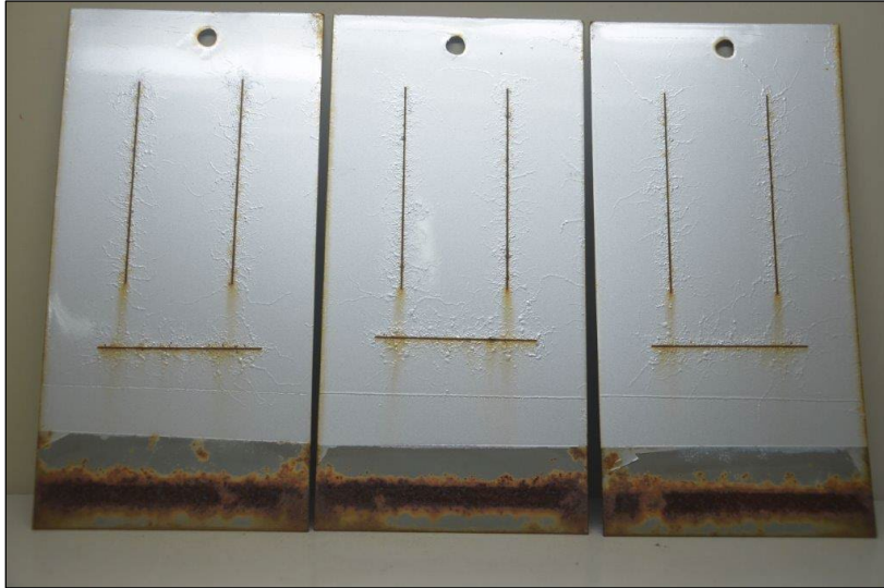
Subtropical Site (not near ocean) Filiform corrosion
