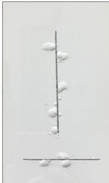
Corrosion morphology – Type D
