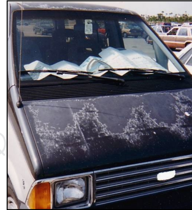
Fading, cracking, peeling
