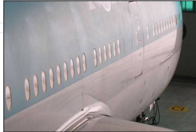
Fading, cracking, peeling
